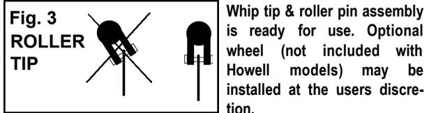
**Once the tip has been aligned, tighten the thumb screw on the whip base only enough to prevent the whip from lifting out of the base. Overtightening may damage the fiberglass strand and integrity of the whip.**
