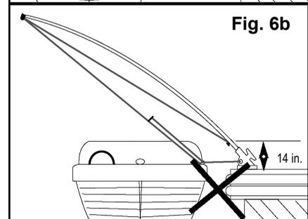
Under no circumstances should any mooring whip be installed with an excess of tension as shown in these diagrams. Doing so will affect the mooring whips ability to protect your water craft and will void the manufacturers warranty.
